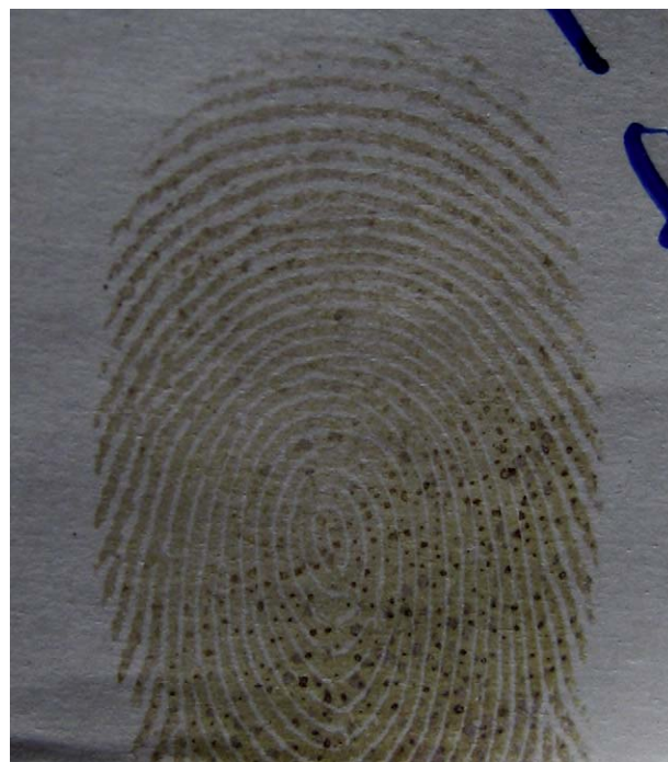
Fig. 7. Fresh latent fingerprint developed on 1-year-old thermal paper sample by iodine fuming showing clear ridge details.
