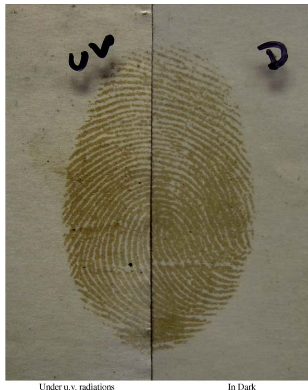
Fig. 3. Fresh latent fingerprint developed on thermal paper by iodine fuming and kept in short UV (left) and in dark (right) for 15 min.
