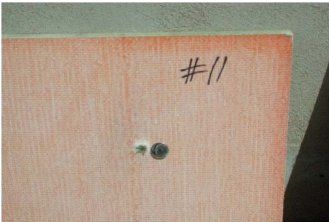
Figure 15. Front side of Kevlar® panel showing bullet entry hole.
