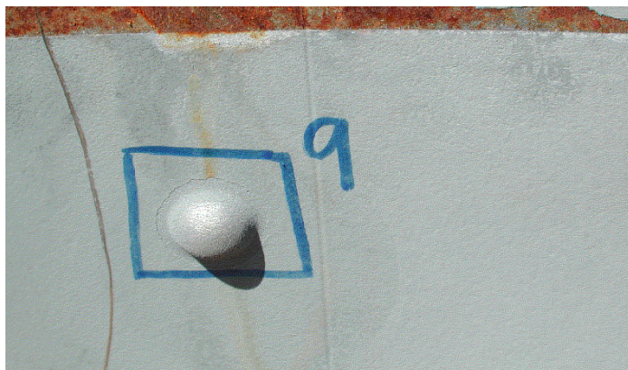
Figure 10. Bullet-induced bulge on back side of steel corresponding to impact crater.
