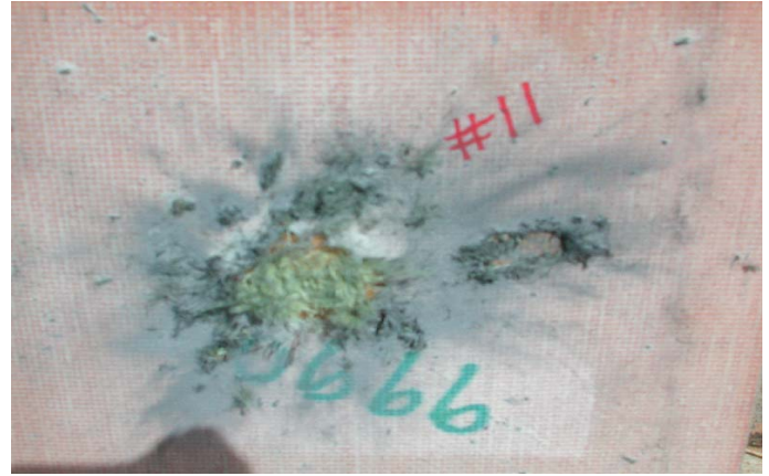
Figure 16. Back side of Kevlar® panel where bullet exited.
