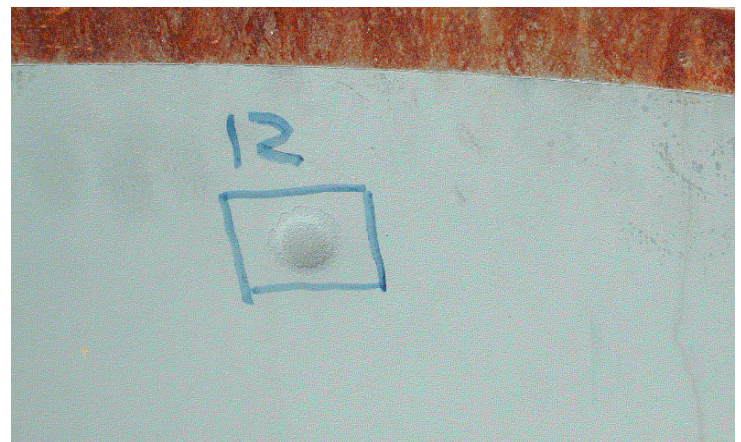
Figure 13: Back view of crater illustrated in Figure 12.
