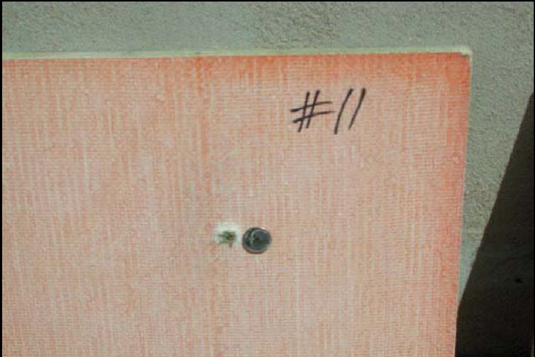
Front side of Kevlar ® panel showing bullet entry hole.
