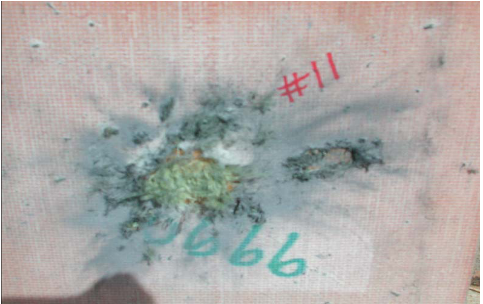
Back side of Kevlar® panel where bullet exited.
